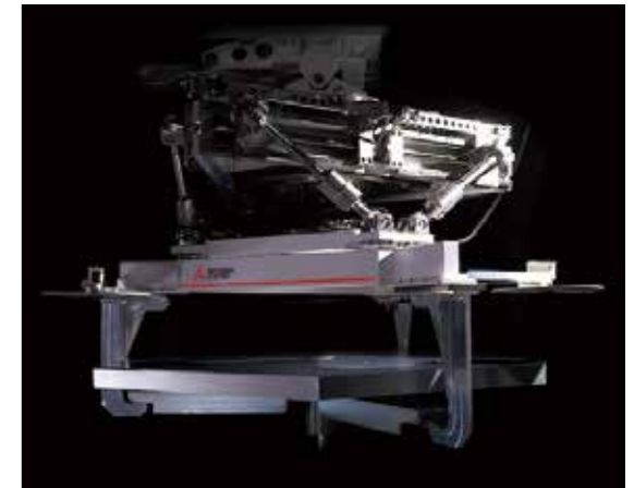
Prototype of a segment-handling robot. In order to keep the highest reflectivity of TMT's primary mirror, 10 segments need to be replaced with recoated ones each day. To ensure swift, accurate, and safe replacement of segment mirrors, the segment-handling robot was devised as an ancillary apparatus. © Mitsubishi Electric Corporation
