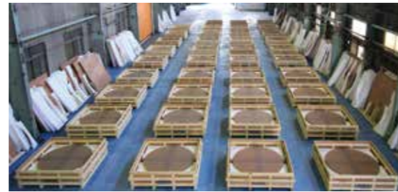
Mass-produced glass blanks for segments of the primary mirror. The segments are being made from Clearceram, a zero expansion glass, so that temperature change overnight will not cause the mirror's expansion or contraction. Segments to be polished overseas are shipped to the US, China, and India when spherically ground. © NAOJ/OHARA
