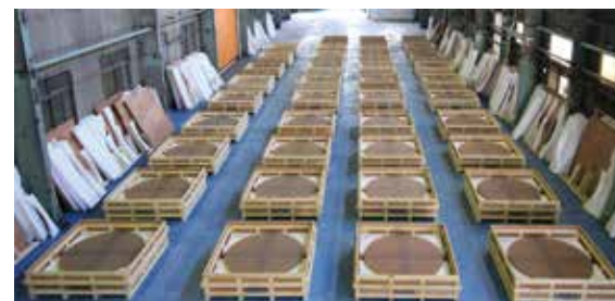
Mass-produced glass blanks for segments of the primary mirror. The segments are being made from Clearceram, a zero expansion glass, so that temperature change overnight will not cause the mirror's expansion or contraction. Segments to be polished overseas are shipped to the US, and India when spherically ground. © NAOJ/OHARA
