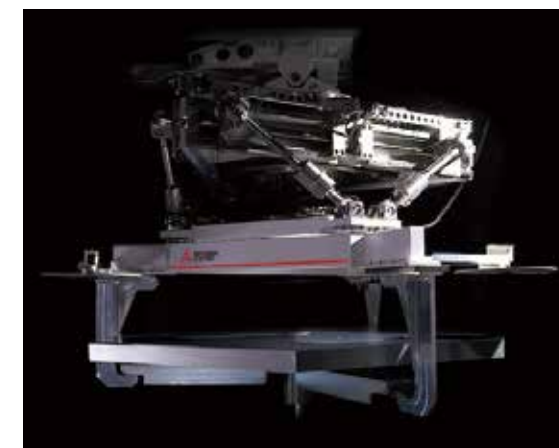
Prototype of a segment-handling robot. In order to keep the highest reflectivity of TMT's primary mirror, 10 segments need to be replaced with recoated ones each day. To ensure swift, accurate, and safe replacement of segment mirrors, the segment-handling robot was devised as an ancillary apparatus. © Mitsubishi Electric Corporation
