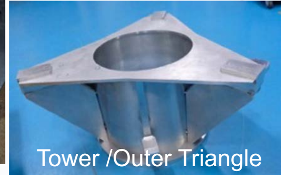
Tower Welding Fixture
