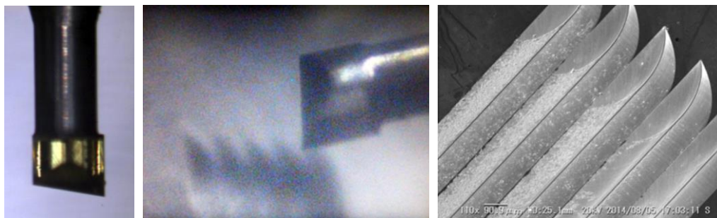
Fig.9 Optical micrograph of tip of end mill of single-crystal diamond (left, \phi=0.5\text{mm} ) and fly-cutting for a silicon substrate (center). SEM image of V-grooves processed by diamond end mill (right).
